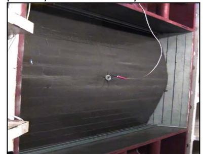
Blast experiment of POSS-polyurea retrofitted concrete masonry unit.
